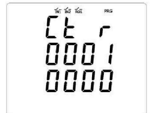
Current Transformer Ratio
