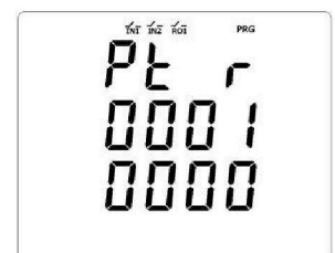
Potential Transformer Ratio
